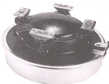
25 PSIG YIELD PRESSURE MOUNT TO 20" PAF WELD COLLARS HEAVY DUTY CLAMP RING
