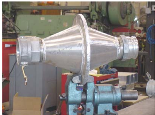
Crunchy-Catcher: stainless steel screen in center to breakdown clumps to speed up unloading
